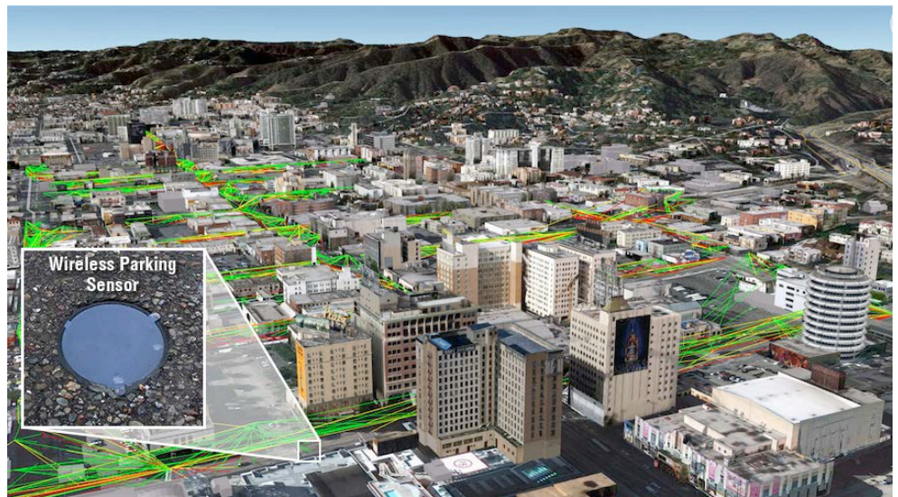
Figure 2. Streetline Networks Has Deployed Time-Synchronized Channel Hopping Networks to Improve Parking in Such Cities as Hollywood, California.
