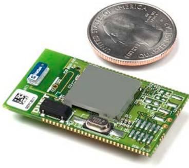
Figure 4. Small TSCH-Based Wireless Nodes, Such as the LTP5901-IPM from Linear Technology, Deliver 5 to 10 Years of Battery Life With >99.999% Data Reliability
