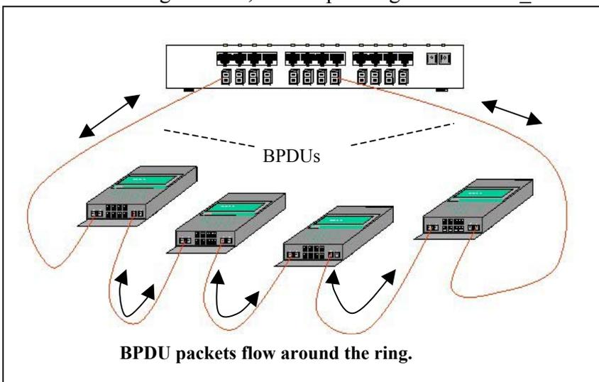
watching the flow of the BPDUs packets that move around the ring between the designated port-pair.
