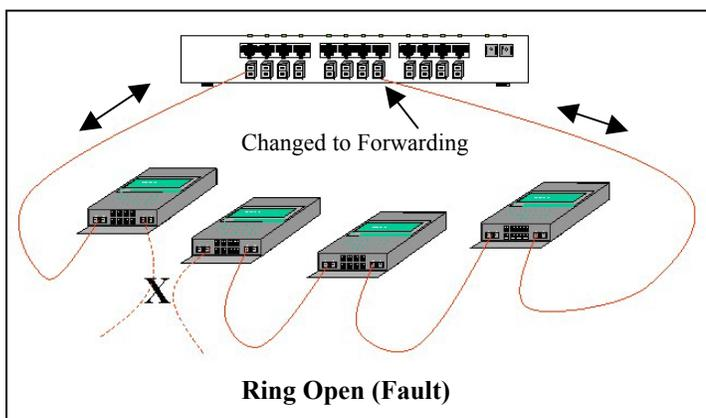
When this change is made by STP and both of the ring manager switch's ring ports are forwarding, the fault is effectively bypassed and there is a path for all LAN traffic to be handled properly. This abnormal status is designated RING\_OPEN, and may continue indefinitely, until the ring fault is repaired. At that time, STP will change one of the ring control ports to be a blocking port again.
