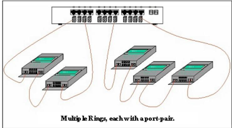
The user, having selected a port-pair for a ring, enables S-Ring on the selected port-pairs via S-Ring software commands. One command (enable / disable) turns S-Ring on and off. Another command adds / deletes port-pairs. Other commands provide for status reporting on the S-Ring product. The Magnum MNS-6K software package provides for remote operation, access security, Event Logs, and other industry-standard managed network capabilities suitable for industrial applications requiring redundancy.
