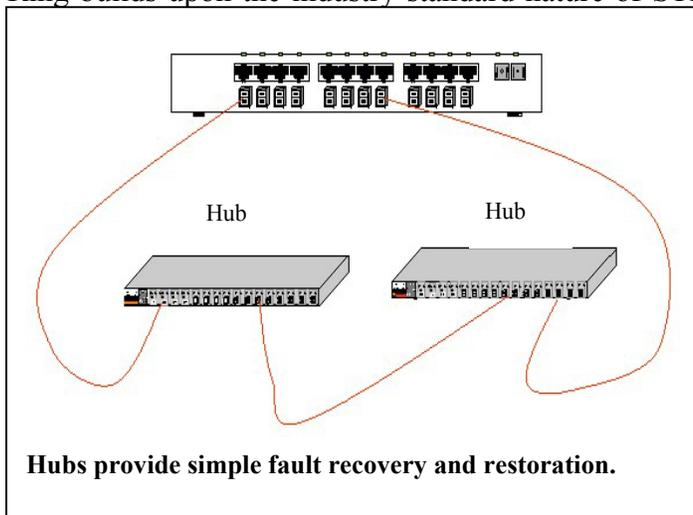
If hubs (repeaters) are used in an S-Ring structure, then the hop-count rules pertaining to Ethernet hubs must be observed. Hubs (repeaters) have no memory and always broadcast each packet. They are easy to re-configure in a ring accordingly. They do not have to change the packet-flow direction when it is time to re-configure for fault recovery and ring restoration.
