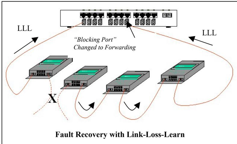
Note that a Link-loss on an mP62 Managed Hardened Switch port somewhere in the ring is an alternative trigger for S-Ring to act for either fault recovery or ring restoration. The interruption (or the restoration) of the flow of BPDU packets is one trigger, Link-loss is another, and action is taken by S-Ring
