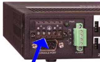
Terminal Block for DC Power
